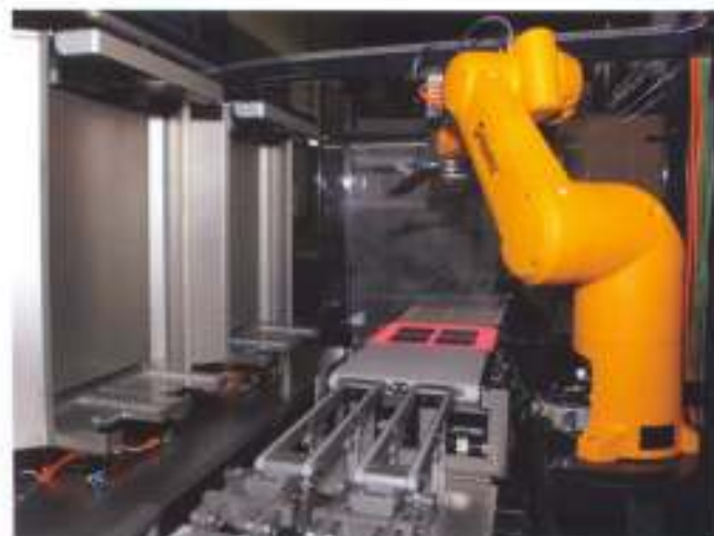
An example of All MEPP engineering: handling system for solar cells.
