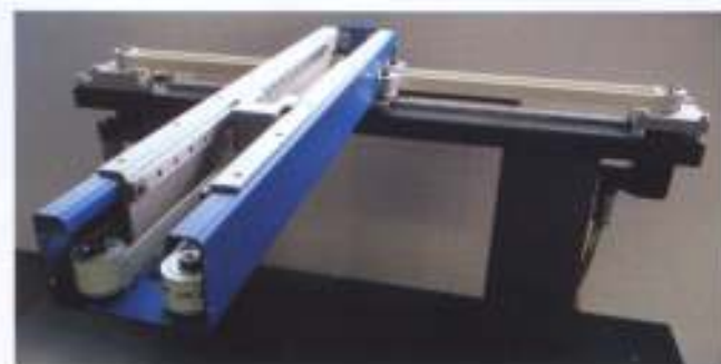
All MEPP's design of a low-cost XYZ system features a measuring range of up to 1,200 mm in all three dimensions.
